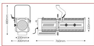
A high efficiency, powerful 200W led module featuring a PWM dimming power source harnessed in the high-specification optics of LDR profile spotlights.
