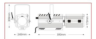
Stylish, compact and extremely high efficiency 100W led wide angle profile spotlight featuring double-condenser optics and a PWM dimming power source
