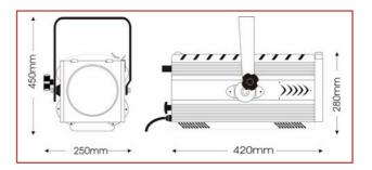
A high efficiency 230W led module featuring a PWM dimming power source harnessed in the high-specification optics of LDR pebble-convex spotlights.
