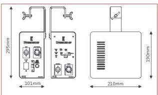
DMX512 / RDM signal and power supply unit for the control of the LDR Xpress range of colour scrollers and most other scrollers on the market.
