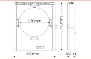
The Xpress 26, DMX515/RDM controllable scroller, is designed for use with those 2000W LDR fixtures featuring a 245x245mm/9.64x9.64 in colour frame or any luminaire with a front aperture up to 270mm (10.62 in).
