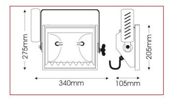
Stylish and high specification 150W asymmetrical discharge floodlight, ideal for usage in all those architectural, display and retail areas applications where a powerful yet low consumption and long lasting beam of light is required.
