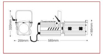
The wider-angle Suono D profile spotlight has a variable zoom focus from 20° to 40°, making it suitable for short-throw applications. The 250W MSD lamp produces a high-power 'daylight' beam which is popular for display, retail and architectural lighting.
