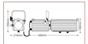
The power of a compact 150W discharge lamp is harnessed by this stylish narrow-angle doublecondenser profile spotlight to project a crisp evenlydistributed beam for highlighting or projecting patterns or advertising logos for architectural and display applications.
