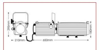
Ideal for display highlighting, this 10°-28° profile spotlight uses a compact 70W discharge lamp combined with a double-condenser optical system. The cool beam design enables a wide range of metal, dichroic or acetate gobos and slides to be used to project images in architectural applications.
