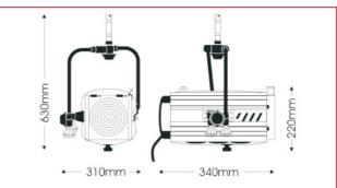
High power discharge Fresnel spotlight for display and internal architectural lighting applications. Suono f250 uses a 250W MSD lamp and produces a soft-edged beam with a variable beam angle ranging from 7° to 63°.
