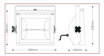
Also for larger venues, this 1000W symmetric floodlight produces a wide, even wash of light for general lighting purposes. Each unit is complete with a safety glass and a double microswitch interlock for safe lamp replacement. The modular design enables several units to be coupled together to form a compartment batten. A colour frame, safety glass and 1.5m mains cable is included as a standard.
